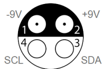
Probe's power supply pin assignment “cable view”
