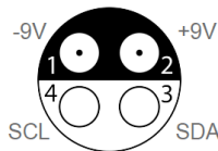
Probe’s power supply pin assignment “cable view”
